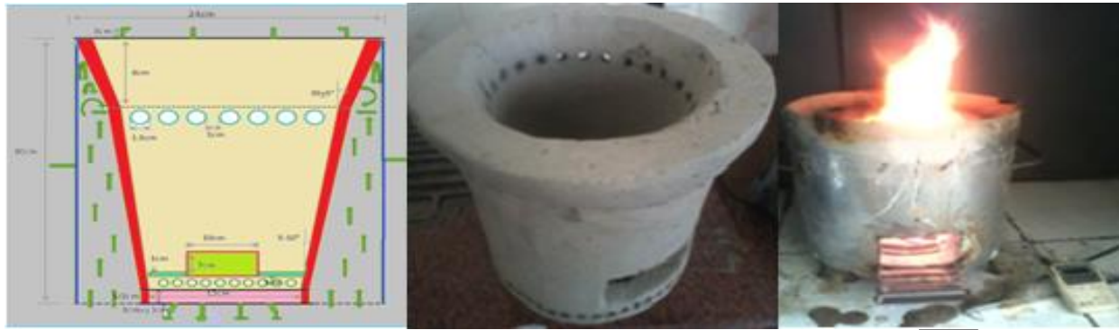
Fig. 5.1 Design Process of Biomass Cook Stove
